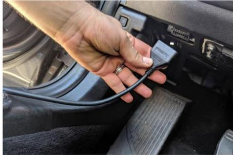
**Figura 2.** Cable conector OBD II.
